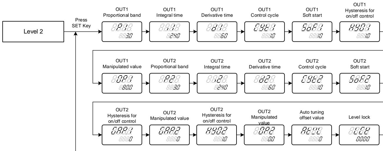
※ : This instrument returns to the PV/SV display mode if no key operation is performed for more than one minute.
