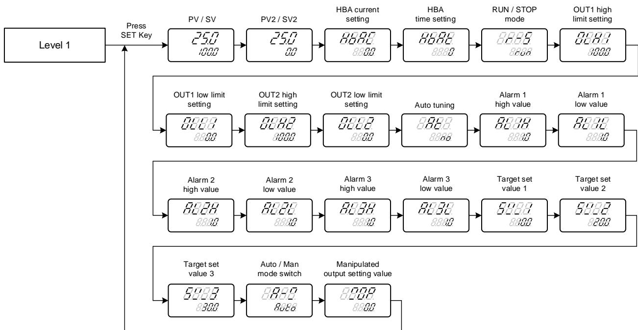
※ : This instrument returns to the PV/SV display mode if no key operation is performed for more than one minute.
