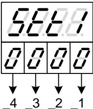
The diagram shows a 4-digit display with four digits labeled \_4, \_3, \_2, and \_1 from bottom to top. Below the display, arrows point downwards to these labels, which correspond to the row numbers in the tables below.
