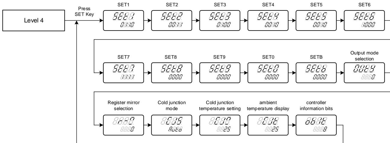
※ : This instrument returns to the PV/SV display mode if no key operation is performed for more than one minute.
